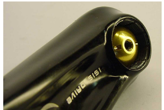
Picture 12: Check crankarm for sufficient space for gear shift button
