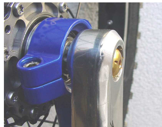
Picture 6: Gear shift button is flush with the crank
