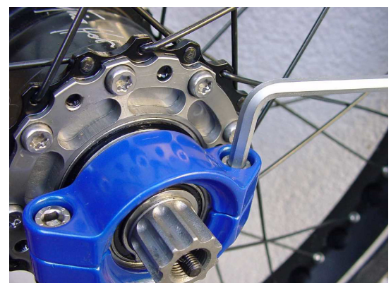
Picture 4: Tighten the screws evenly with 5-6 Nm!
