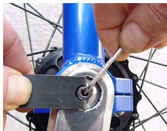
Picture 7: Hold the gear shift button with the black wrench and tighten it well with an 2mm Allen wrench
