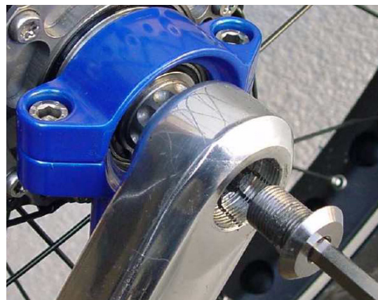
Picture 5: Mount crankarm and adjust axle bolt
