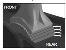
Saddle angle is easily adjusted by loosening the Pivotal seatpost bolt through the top of the saddle. Use the number of Pivotal "steps" visible behind the seatpost as a reference. The saddle has a 24° adjustment range in 6° increments.
